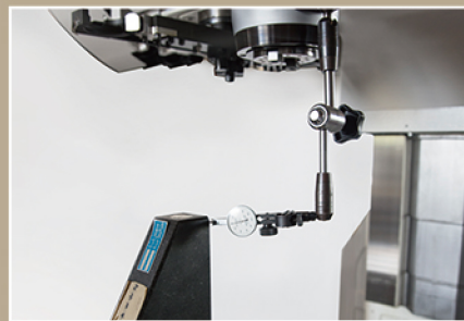
Vertical straightness of Y&Z axis
