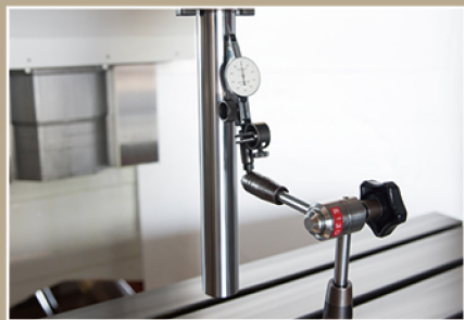
Spindle run-out check
