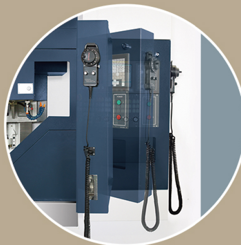
Built-in type operational box with 120° adjustable rotary arm.
